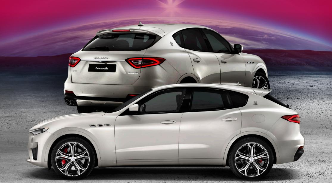
sends power to all four wheels using Maserati's Q4 rear-biased all-wheel-drive system, which includes a mechanical limited-slip differential on the rear axle that can lock up by 25 per cent under power and 35 per cent under release.
