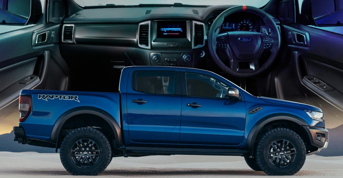
Compared with current range topper, the Wildtrak, the Raptor is 330mm wider (2180mm), and sits on a track widened by 150mm at each end. It is also rides 25mm taller at 1873mm and 9mm longer at 5398mm.
